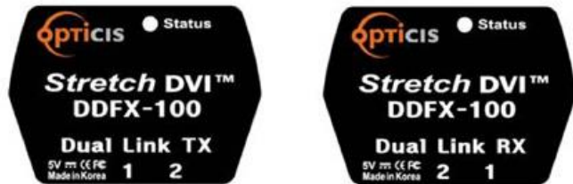
Figure 2 – Fiber numbering and Status LED position on a label
